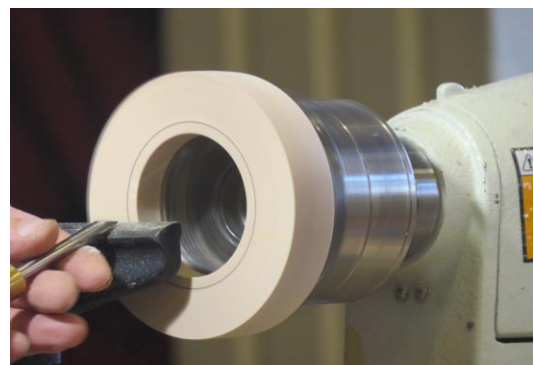
Reversed onto large jaws and cut inset for photo, etc.
