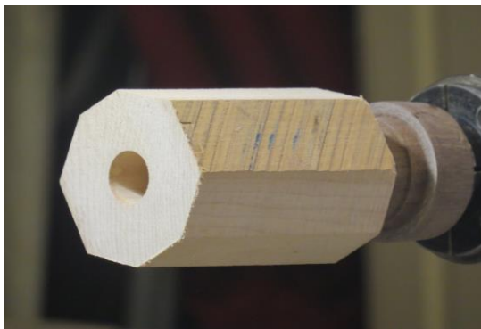
Body drilled for grinder mechanism
