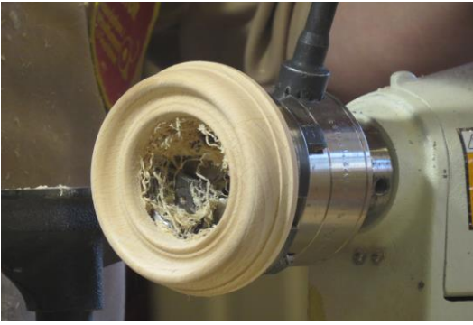
Reverse on jaws and shape the face of the frame
