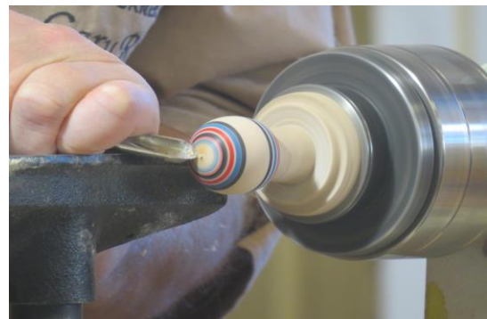
For the spinning top to work correctly the base must be given a slightly flattened shape
