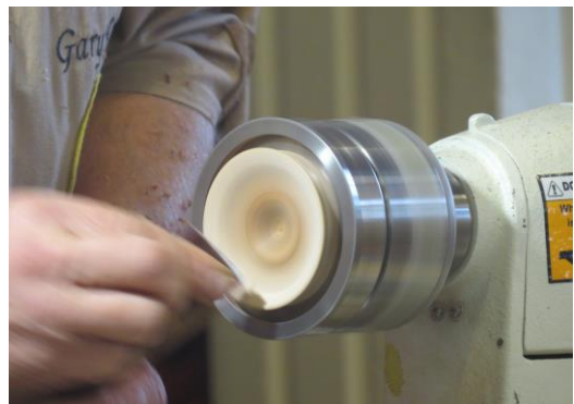
In jig, turn one side then the other side.
