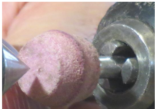
Small grindstone shaped to form groove on the plum
