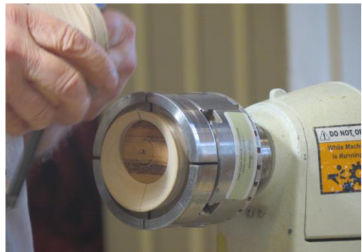
In jig, turn one side then the other side.
