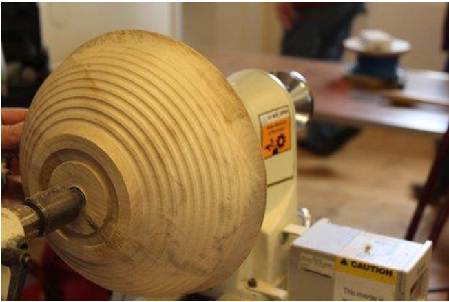
another consideration, coves cut with negative rake tool
