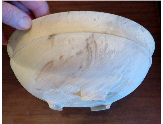
Final shape showing rim detail and shaped feet
