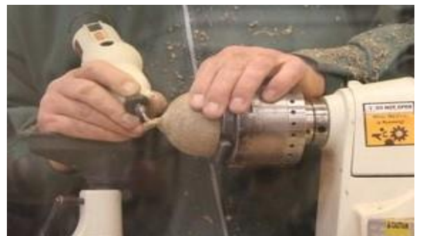
Texturing the cup with a globe burr cutter
