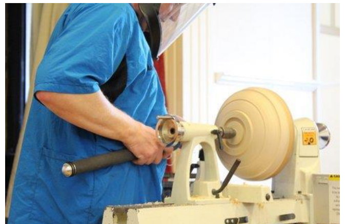
Forming shape showing the base inset and spigot
