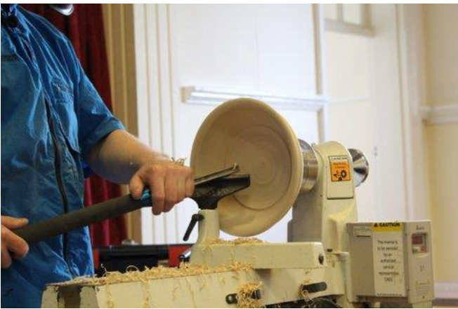
another consideration, coves cut with negative rake tool
