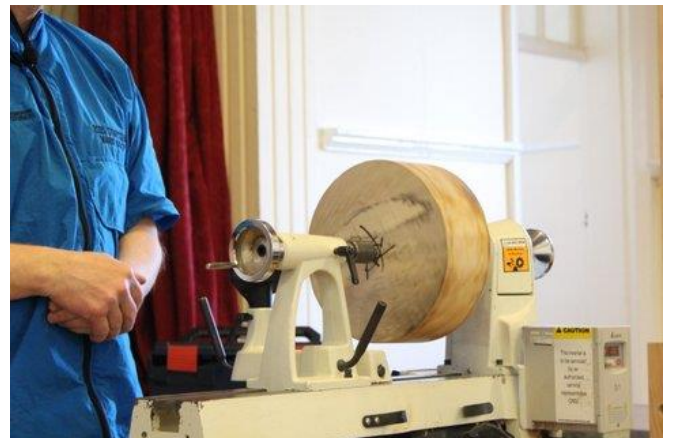
Sycamore blank between centres
