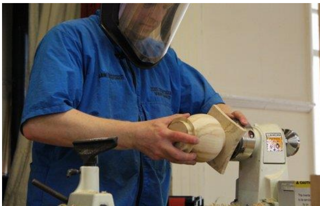
checking the fit of the square lid
