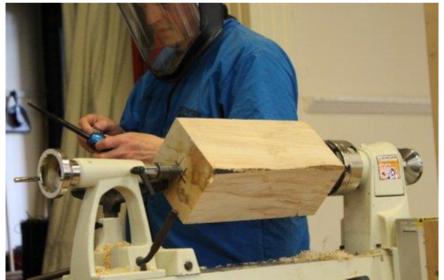
between centres turn to round and cut spigot
