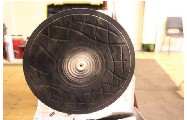
Ebonising spray applied as a base colour
