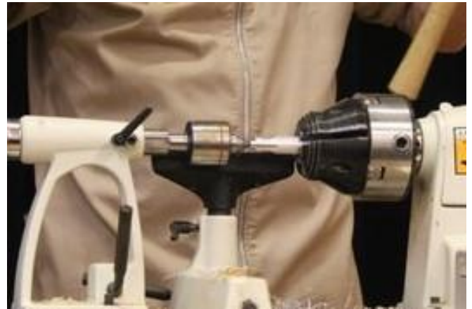
Carefully shaping the aluminium stem
