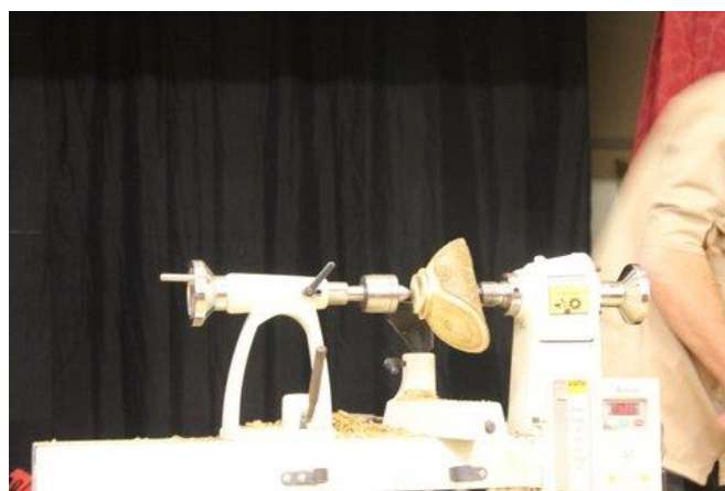
Shaping the base and preparing spigot
