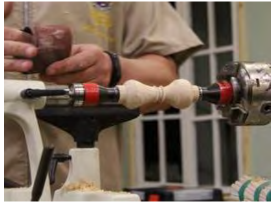
Separate the glues joint, sand the back and round over the ends.
