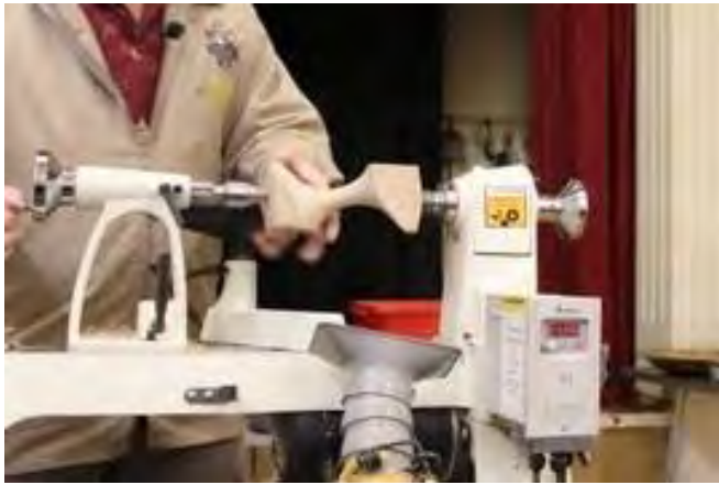
Remount on centres and finish the base.
