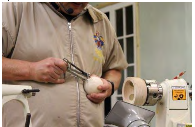
Using a Jacobs chuck drill a hole for the eye.
