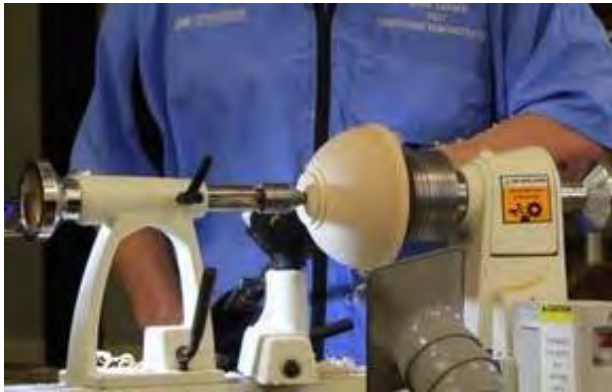
Hollowing - drill out to depth using a colt forstner bit with an extension rod as required.
