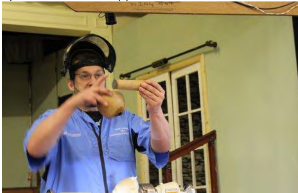
Reverse mount to finish the base by placing a scrap cylinder inside to support it and then the tail stock.
