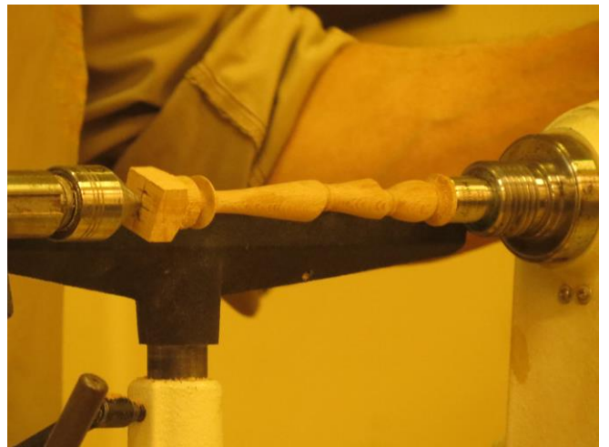
Finally - some off-set turning
