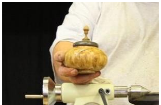
Finished with sanding sealer and microcrystalline wax
