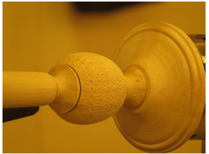
Detail of the texturing – applied with Sorby texturing wheel
