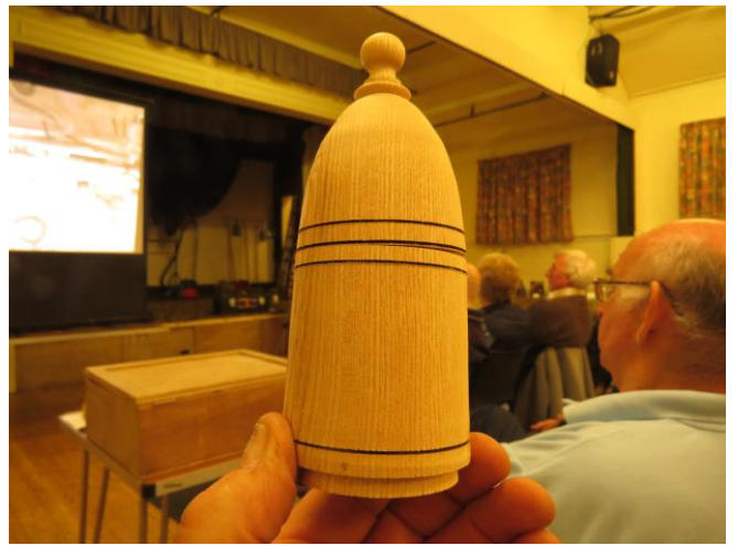
Almost complete - apart from removing the base spigot and applying a finish
