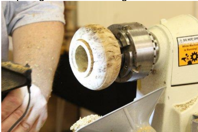
Hollowing out the box
