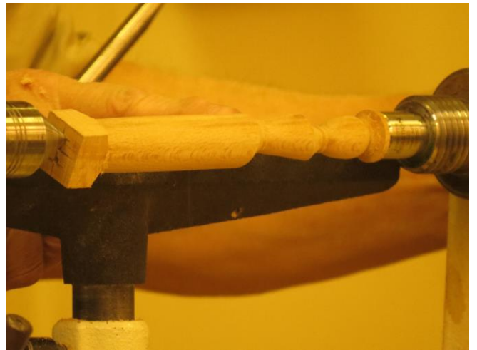
Finally - some off-set turning
