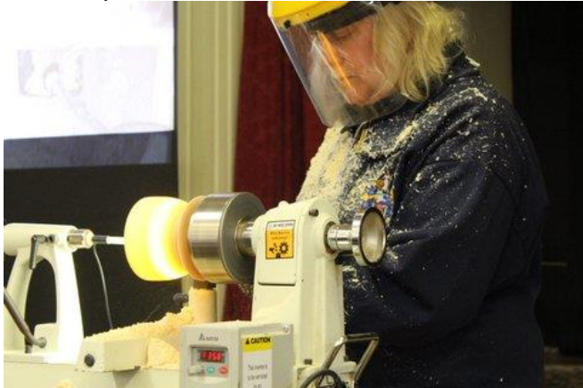
Forming the basic thin walled bowl from wet sycamore – using a light to judge even wall thickness.
