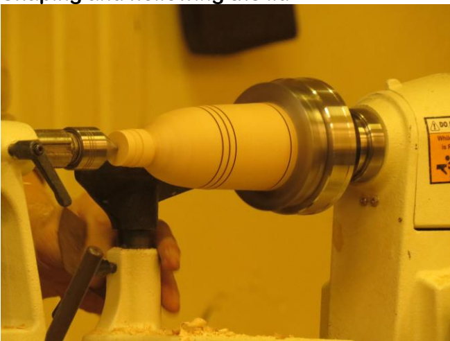
Shaping the finial
