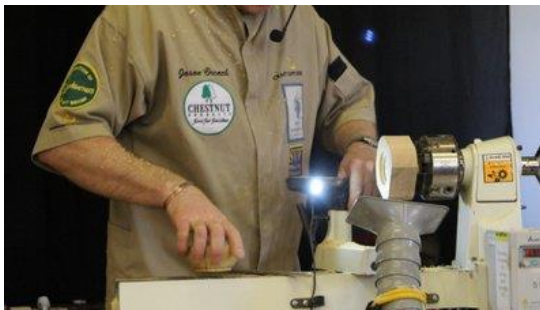
Making jam chuck to remove spigot on the base.
