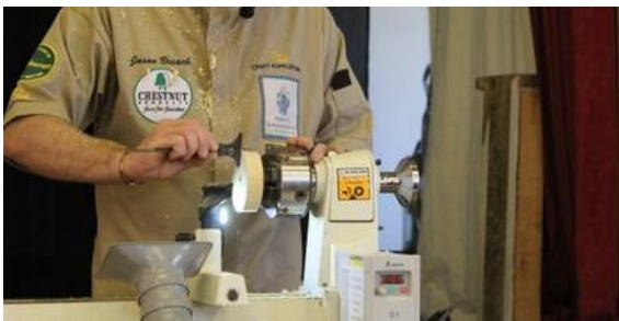
Lid parted off 1/3 of length – spigot in jaws.
