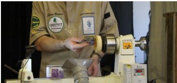
Hollow out lid to dome shape
