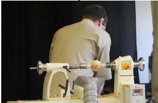
Between nylon centres to remove stubs Ball then placed into jam chuck, a small flat face formed. Forstner drill to depth of 10mm. A further small flat cut at an angle to the hole. Clock fitted into drilled hole.
