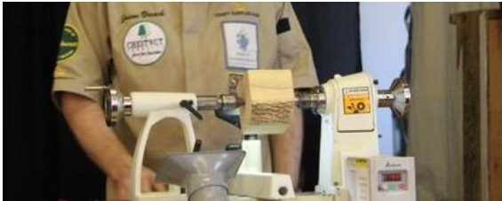
Boxwood turned to round between centres And spigot formed at each end.
