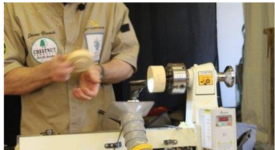
Body in chuck being hollowed out.
