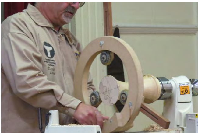
Custom made steady being fitted prior to hollowing out.
