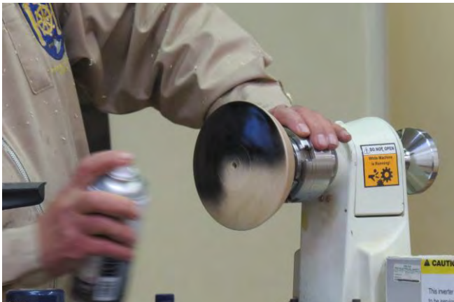
Paint being applied following an application of sanding sealer
