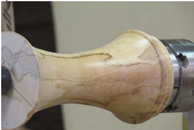
Turned to shape and polish applied.
