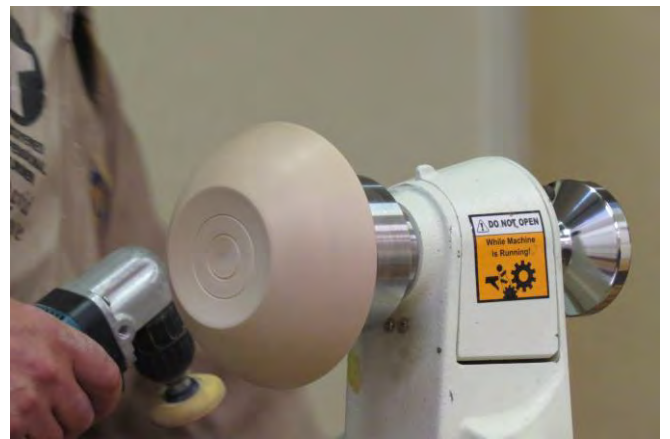
Chucking point removed and base completed.
