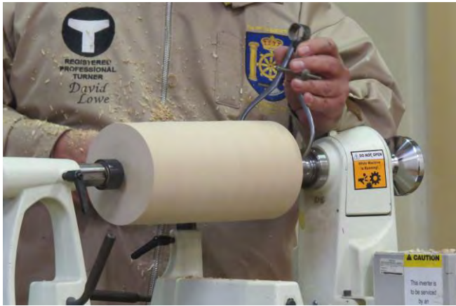
David turned to round a significant piece of sycamore between centres.
