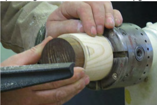
Ensure the grain direction of the insert is in line with the base wood. Glue in with CA glue.
