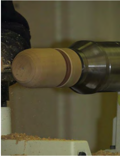
Forming the apple held in a screw chuck
