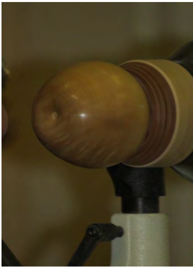
Forming the apple held in a screw chuck
