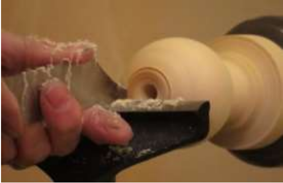
Marking the insert diameter with a thin parting tool.
