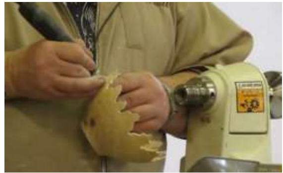
Using high speed drill to cut out the rim
