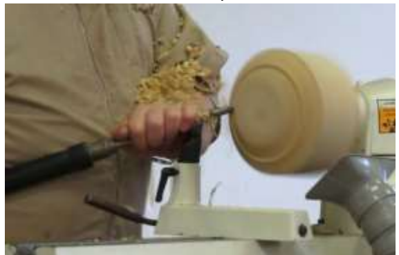
Forming the external shape
