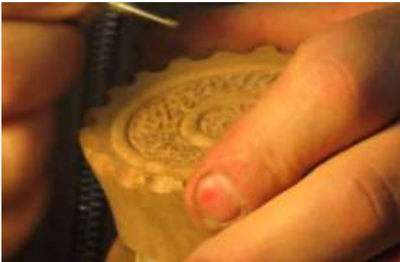
Random texturing formed with high speed ball shaped milling tool
