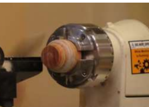
Jam chuck from scrap wood
