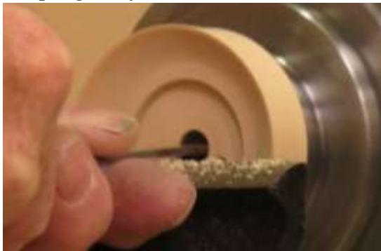
Refining the cup for the lighting assembly
