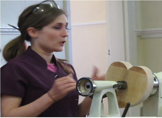
Mounted between steb centre and revolving tail centre
