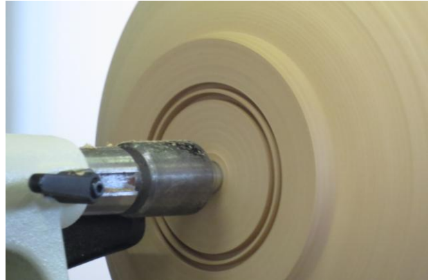
Forming the spigot for reverse turning
