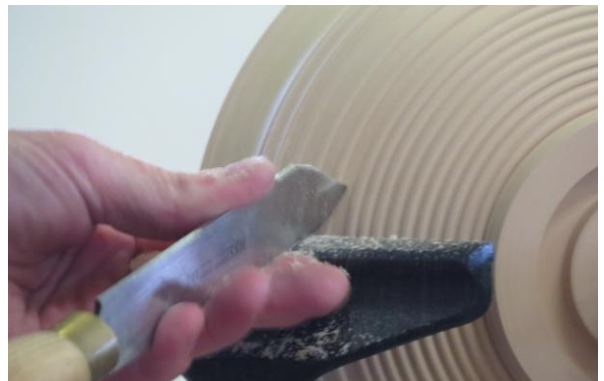
Removing alternate beads with parting tool
