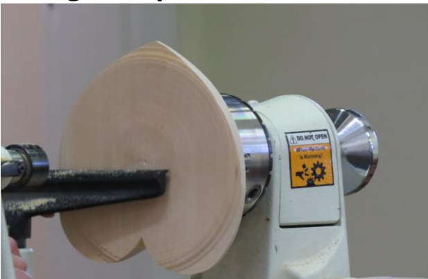
Mounted on jaws the top face is shaped, ensuring sufficient wood is left to carve the ripples
