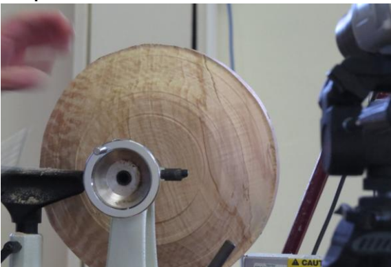
Outside being formed between centres
