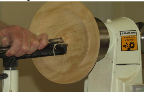
Shaping the underside of the lid
