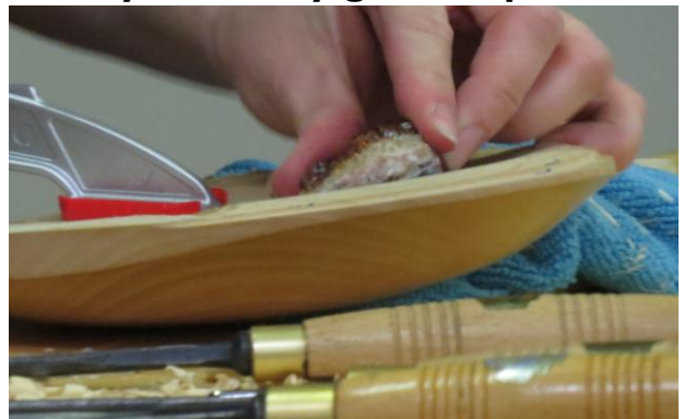
Chalk used on the back of crystal to indicate the areas to carve for a good fit. Crystal finally glued in place.
