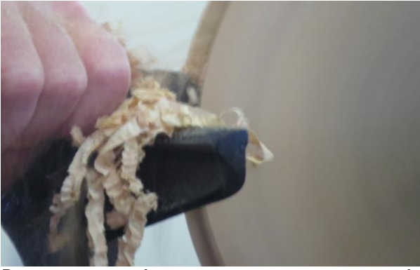
Removing the centre core with a McNaughton Centre Saver
